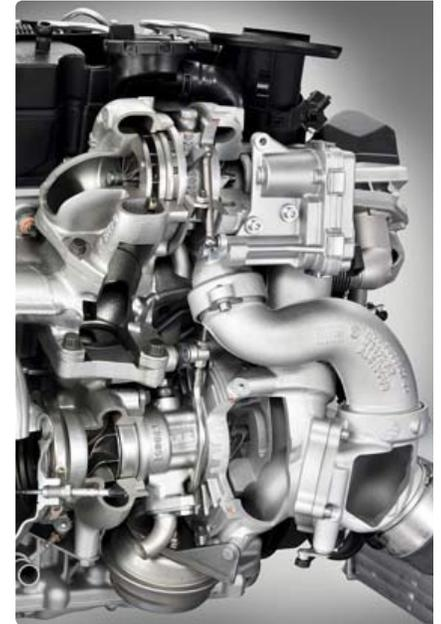
ing 75% of its maximum torque from just 1,000 rpm. Once the small turbo reaches the limit of its throughput, the larger turbo then takes over and secures plentiful power delivery at higher revs from the inline 6-cylinder engine.
